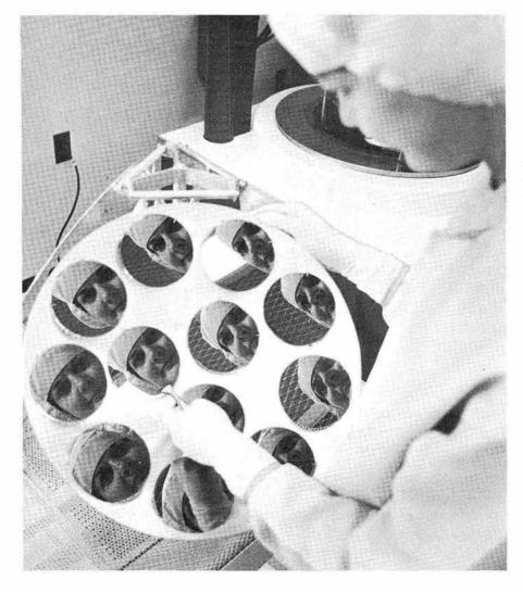
WAFER, WAFER on the wall, which will become the base for a radiationhardened large-scale circuit? The answer, says technician Judy Odinek (2141), is darn near all. She's loading the silicon wafers prior to the next step—metal deposition in the vacuum furnace. Photo was taken in Sandia's Semiconductor Development Lab.
